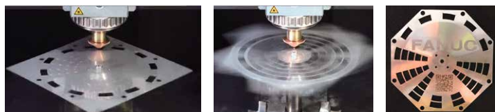
High-speed, high-precision cutting and marking of rotating workpiece ("FANUC" character marking)
