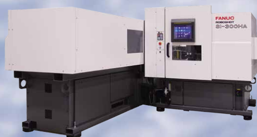
Horizontal second injection unit ROBOSHOT SI-300HA
