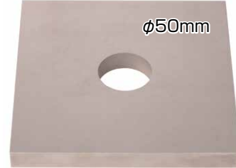
Die steel, 20mm 1 rough 5 skims Roundness 0.90μm
